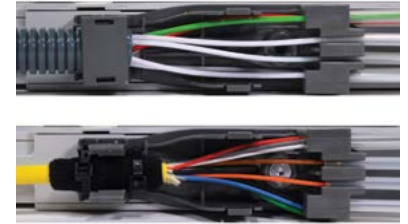
Figure 19: Installed cable termination units (CTUs) on FACT chassis
