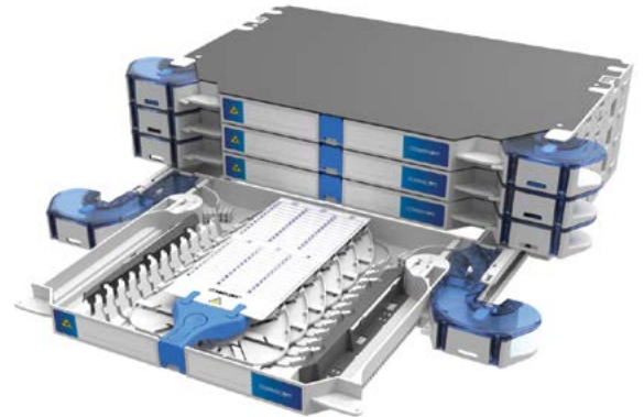
Figure 20: Four-element splice chassis, six trays per element, 12 SMOUVs per tray
