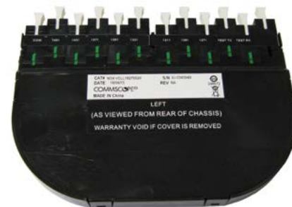
Figure 16: CWDM, 8 channels + T, with SC APC connectors
